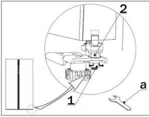
Open the door, loosen the locknut (1) with a wrench (a)..
